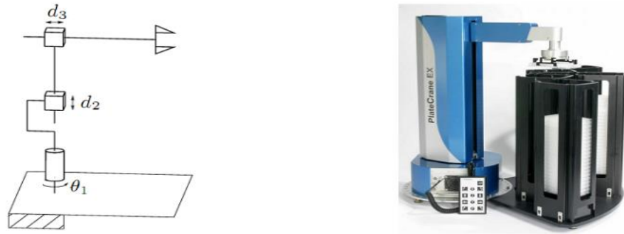
Figure 4 :illustration de la structure cylindrique [16]
