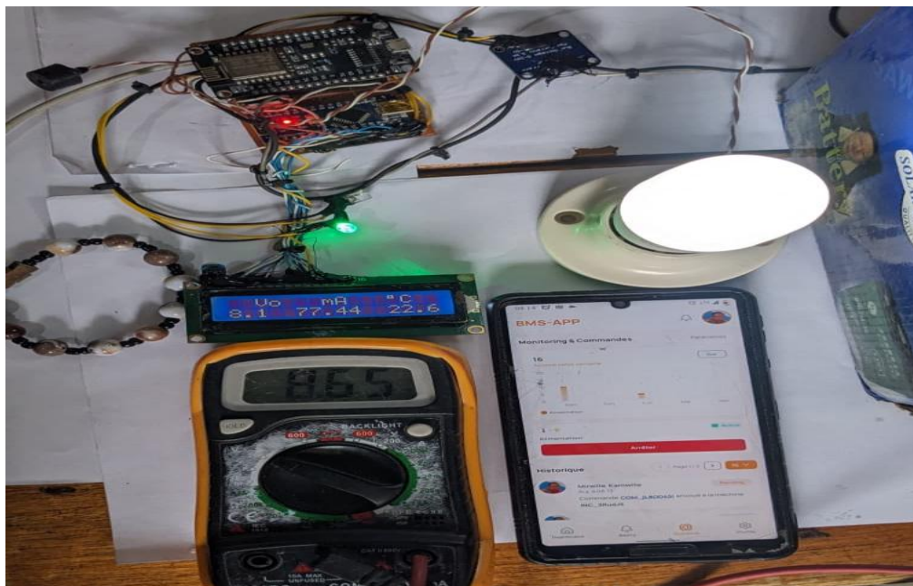
Figure 26: Photo du banc de test complet (batterie + BMS + instruments)
